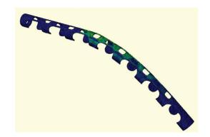
**Figure 8.** Nickel-titanium based shape memory alloy (SMA) alternates between a flaccid and erect configuration with application of heat. Source: Le *et al.* [2013].
